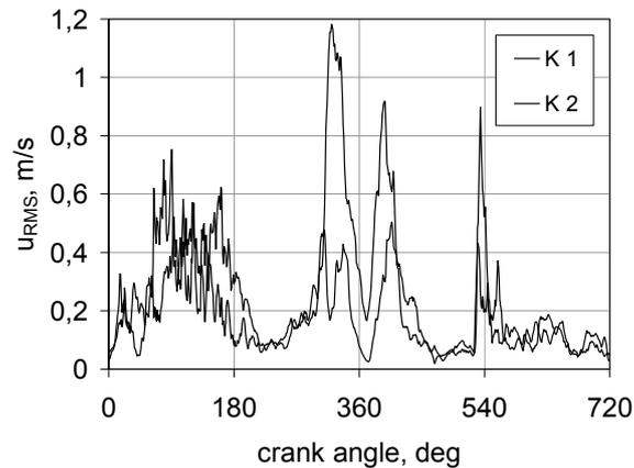
Fig. 8. Velocity fluctuation for two perpendicular directions
