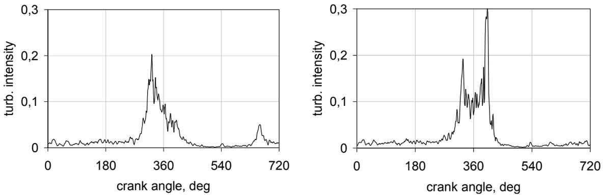
Fig.4. Turbulence intensity variation curve in ignition points
