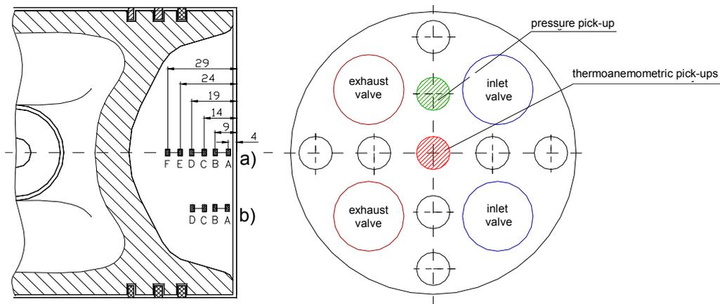
Fig. 2. Configuration of measurement points in combustion chamber of research engine.
