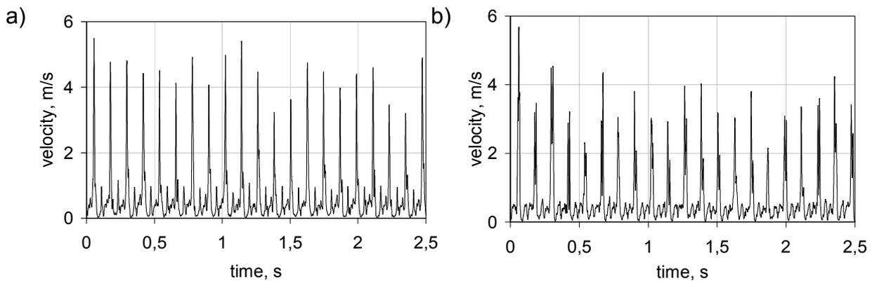
Fig.3. Charge instantaneous velocity variation curve in the ignitron points of the research combustion chamber
